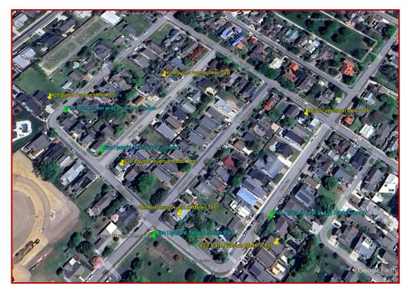
Six (6) samples were taken from existing water meters, and four (4) samples were taken from existing fire hydrants in the vicinity. The results of the Envirocorp Laboratories, Inc. iron concentration testing are summarized in the tables below.
