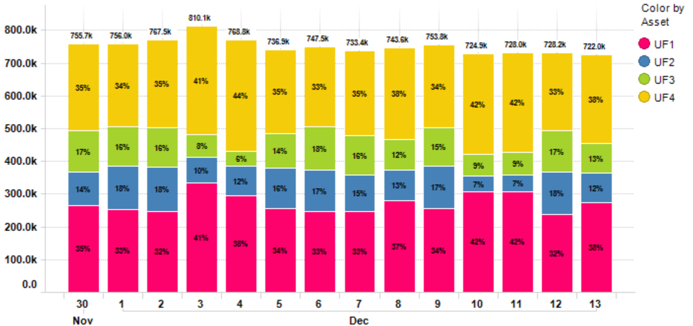
Average Daily permeate flow from 11/30/2022 to 12/13/2022 is 748.3k gal with a maximum daily flow of 810.1k gal.
