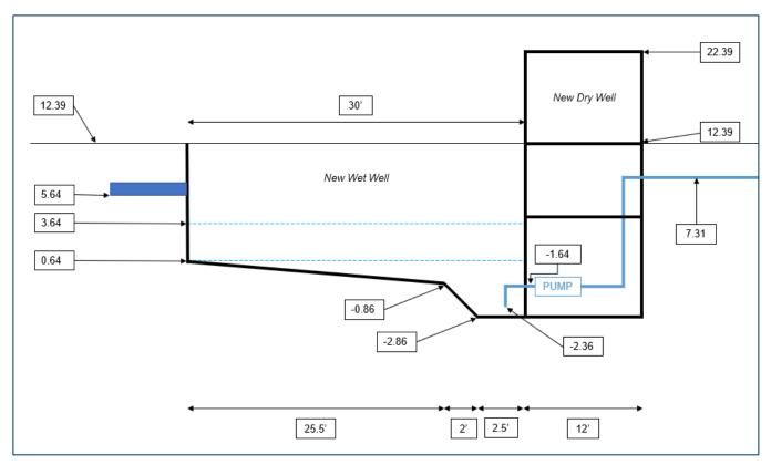
Figure 26 Options 2b/c, Treated Effluent Pump Station Schematic (Section)
