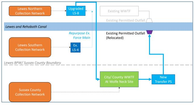
Figure 29 Option 3a, Network Schematic
