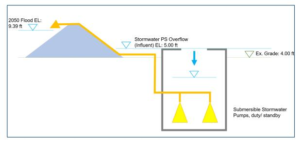
Figure 16 Option 1, Stormwater Discharge Pump Station Concept Arrangement, Section View
