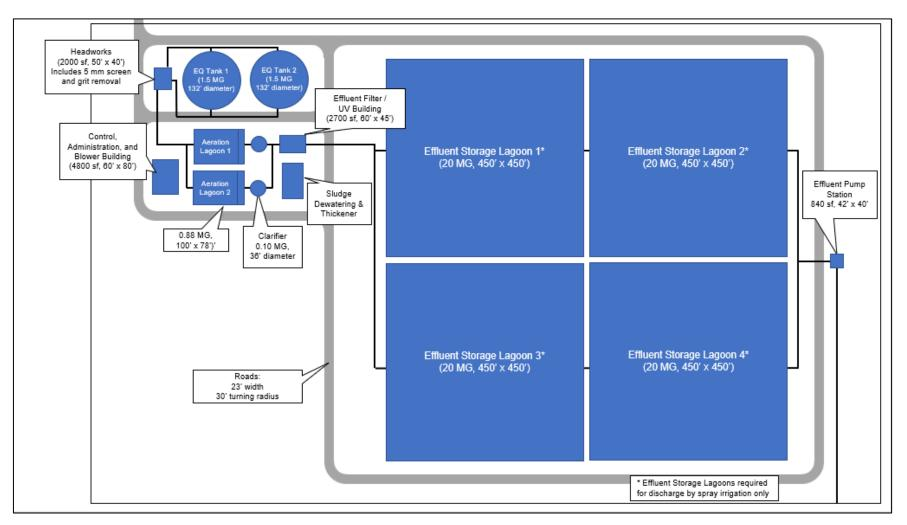
Figure 20 New WWTF Schematic Layout, Activated Sludge Treatment Process with Effluent Filtration
