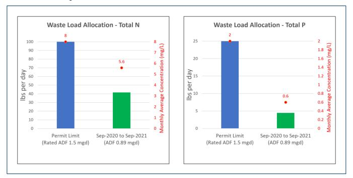
The estimated average effluent waste loads for Total Nitrogen (TN) and Total Phosphorus (TP) during this time period are summarized in Figure 5.
