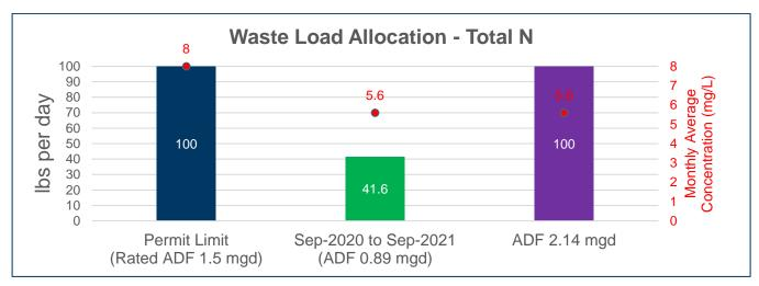
Figure 6 Comparison of Existing Effluent Waste Load Performance Compared with Permit Limits, Total N
