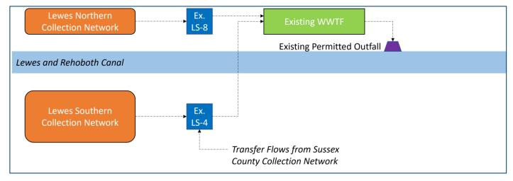
Figure 2 Existing WWTF Flow Schematic
