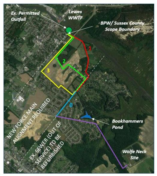
Figure 32 Option 3a, Potential Treated Effluent Force Main Alignment Alternatives
