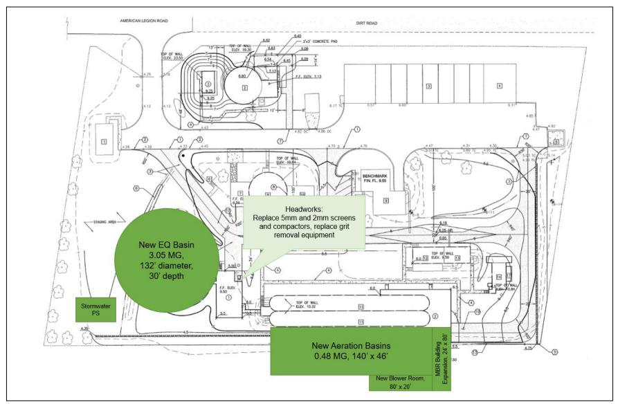
A schematic layout showing the process upgrades required for Option 1 is provided in Figure 12.
