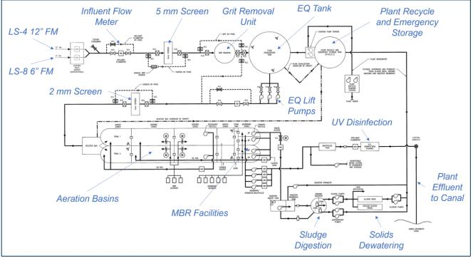
Figure 3 Existing WWTF Flow Schematic
