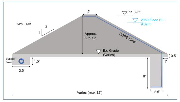
The flood barrier system would be composed primarily of compacted fill; a typical section through the compacted fill barrier is provided in Figure 14.
