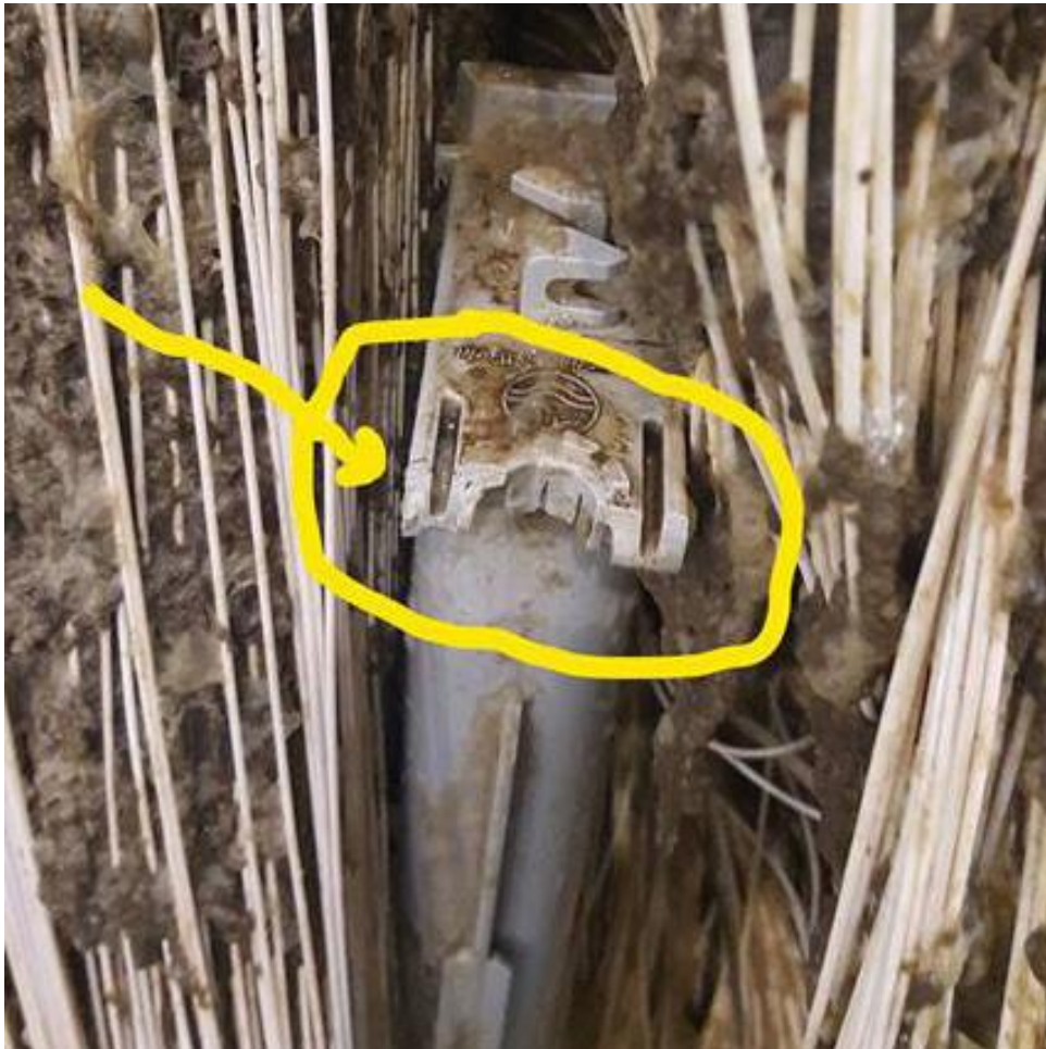
Picture 4 – Lower Lock Tab Break and dislocated header, April 2019
